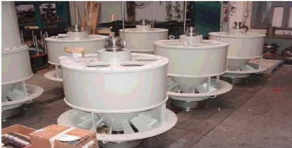
Figure 9: The six axial propeller turbines being assembled at Kössler GmbH (left) and one of the turbines being installed on the prototype in the open sea (right).
