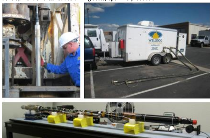
Figure 4. SweetSpotter 3" downhole tool and truck in the field. Lower picture shows a new downhole tool being built in the lab.
